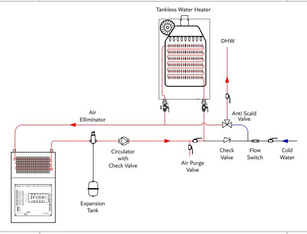
AHU with Tank Water Heater Space Heating Application
