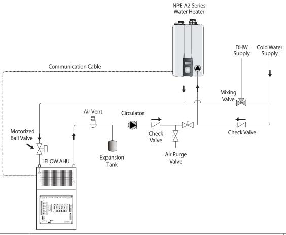
iFLOW AHU & NPE-A2 with External Recirculation
