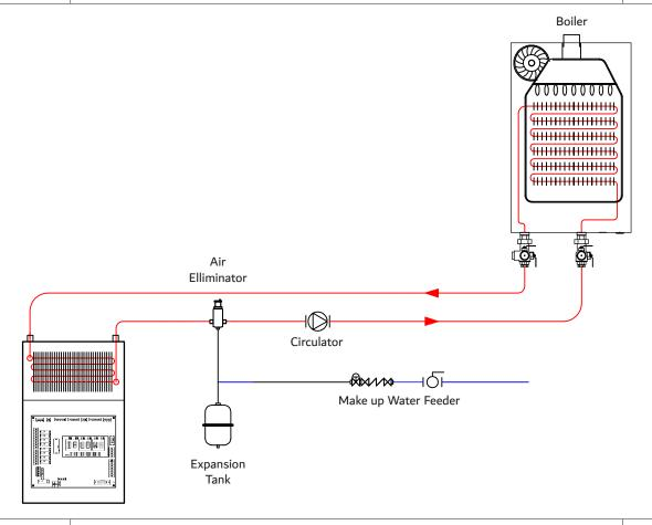
AHU with Combi Boiler Space Heating Application
