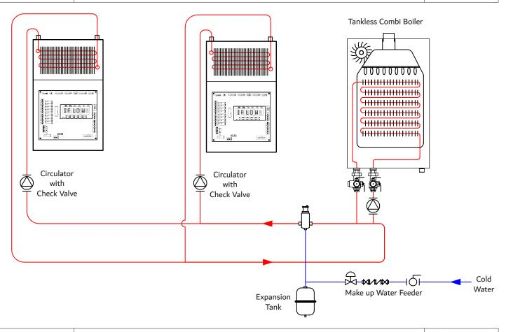
2 AHU with Combi Boiler Space Heating Application
